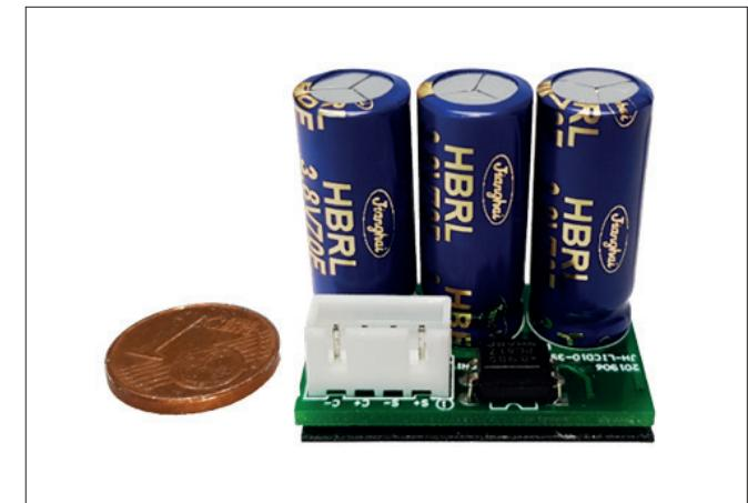
billing systems. So that no data is lost in the event of a power failure or accidental disconnection of the power supply, these must be stored and (computing) processes terminated in a controlled manner. Depending on the application, this type of sudden interruption is not uncommon. A reliable energy storage system is essential for such applications
