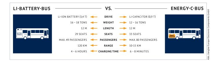
count the mechanical protection required for batteries). This is exactly where the Jianghai engineers start with the new bus concept: They did not try to install ever larger battery modules in order to achieve the longest possible range, but they rather changed the operating mode in order to be able to use capacitors instead of the batteries. Instead of a long term stop at a charging station for several hours, the buses charge their capacitor modules for a few minutes at each stop.
