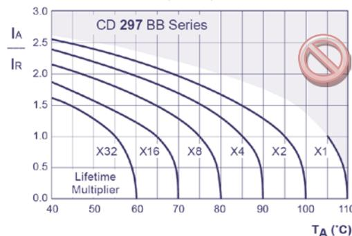
**Fig. 7: Lifetime diagram for Jianghai elcap series CD\_297\_BB**
