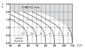
I<sub>A</sub> = actual ripple current at 100kHz,
