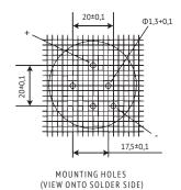
For øD  $\geqslant$  30mm only. For diameter øD  $\geqslant$  45mm the safety vent is typically placed at the side of the housing.
