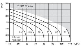
$I_A$  = actual ripple current at 120Hz,
