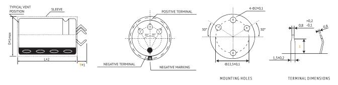
For øD  $\geqslant$  30mm only. Other terminal types and styles on request. For diameter  $\emptyset$ D  $\geqslant$  45mm the safety vent is typically placed at the side of the housing.
