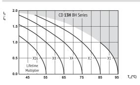
$I_A$  = actual ripple current at 120Hz,
