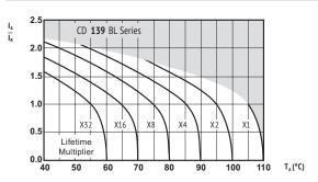
$I_A$  = actual ripple current at 120Hz,
