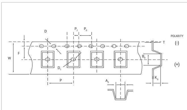
**DISC STRUCTURE AND DIMENSIONS (Unit: mm)**
