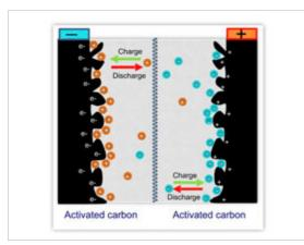
Fig. 2: Electrode structure of EDLC
