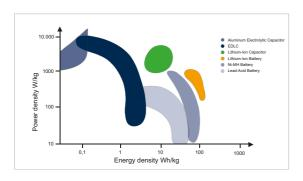
Fig. 1: Ragone diagram of various storage devices for electrical energy
