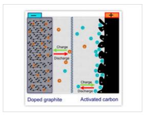
Fig. 4: Electrode structure of Li-C
