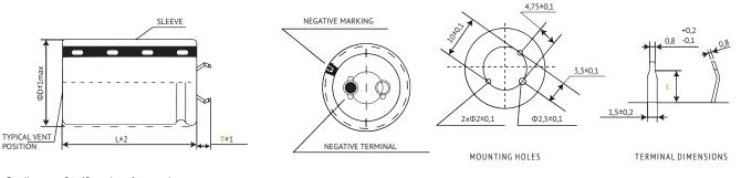
For diameter  $\emptyset D \ge 45$ mm the safety vent is typically placed at the side of the housing.
