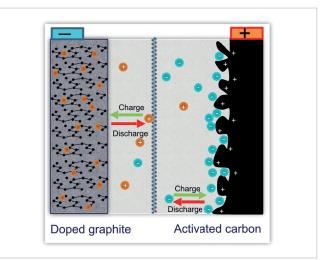
Fig. 4: Electrode structure of Li-C
