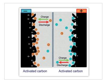
Fig. 2: Electrode structure of EDLC
