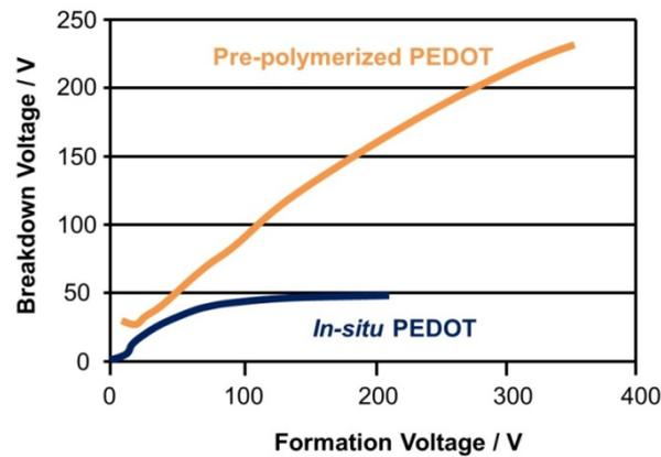
Fig. 5: Process-dependency of the dielectric breakdown voltage [12]
