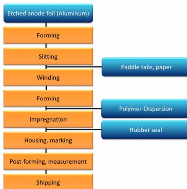
Fig. 6: Manufacturing process of polymer aluminum electrolytic capacitors
