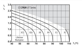
$I_{\rm A}$  = actual ripple current at 120Hz,  $I_{\rm R}$  = rated ripple current at 120Hz, 105°C
