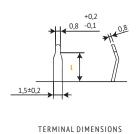
Standard Version: Self-Lock Terminal. Other terminal types and styles on request. For diameter  $\emptyset D \geqslant 45$ mm the safety vent is typically placed at the side of the housing.
