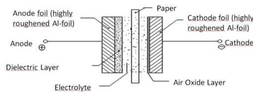
**Fig. 1: Construction of an aluminum electrolytic capacitor**
