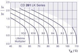
$\rm I_{\rm A}$  = actual ripple current at 100kHz,  $\rm I_{\rm R}$  = rated ripple current at 100kHz, 105°C Multiplier of Useful Life as a function of ambient temperature and ripple current load
