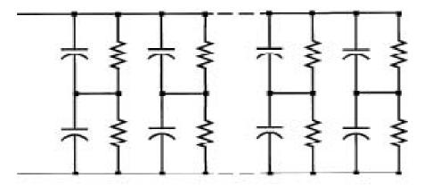
Advantages: If one capacitor fails, the capacitor in series will fail too, but remaining capacitors in the bank are unaffected. If balancing resistors are not used, high leakage current of one capacitor affects only a single pair of capacitors. For safety reason of the application this version is recommended.
